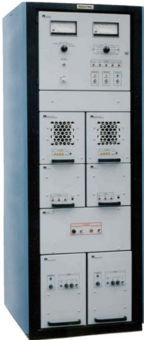
NAUTEL has developed the GPS1000 as an extremely efficient and highly reliable transmitter especially suited for use at remote unattended indoor installations. The 1 kW output is fed via a 50 ohm coaxial feeder directly to a separate automatic antenna tuning unit Type NX4000TUB to a suitable customer supplied antenna.
