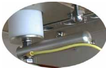
Adjustable Spark Gap and Direct Ground
